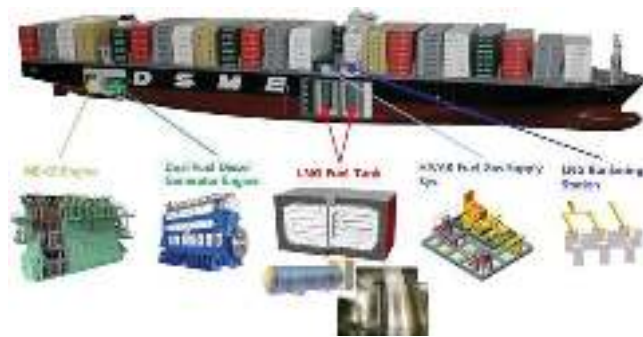
A diagram of the construction of a typical LNG-fueled ship built by the DSME.
